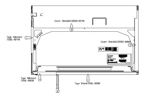
Figure 4-69 Replacing LG.Philips fluorescent lamp (WXGA) (8)
